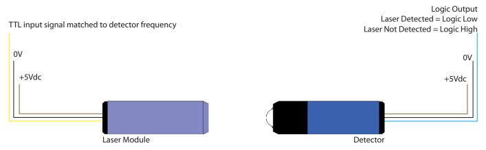
2) Modulating the laser with the output of the detector by connecting the detector and laser third pins (yellow wires) together, the ground references should also be common.
